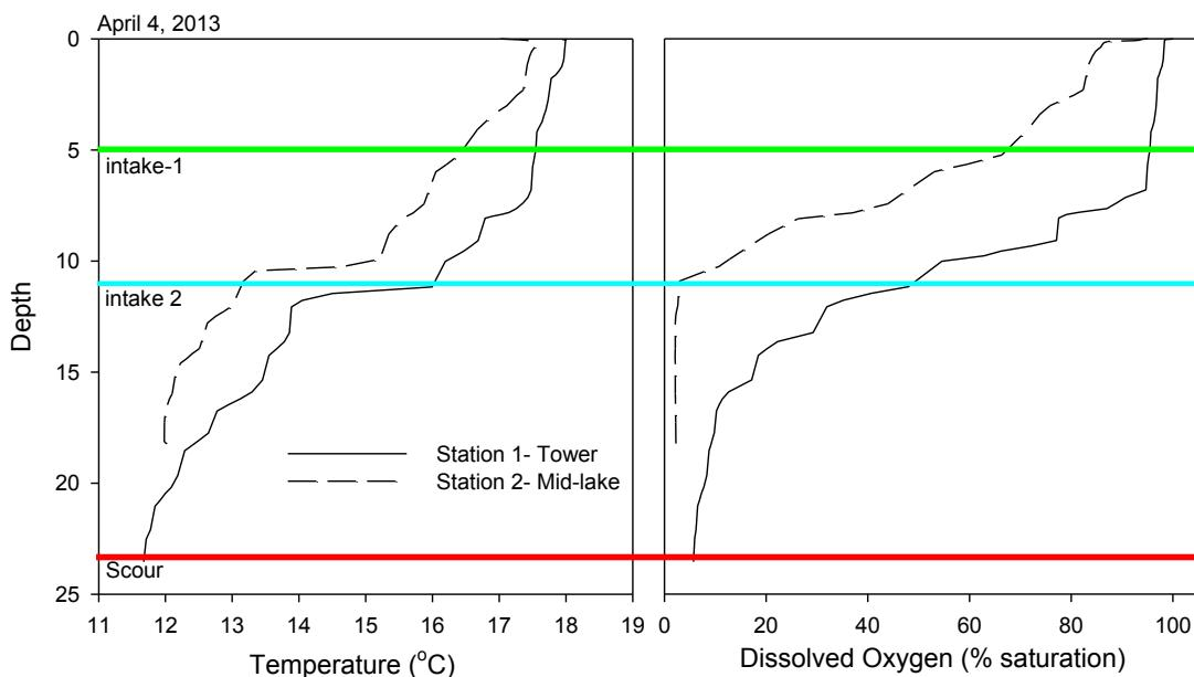
Figure 9. Depth profiles of temperature and dissolved oxygen (DO) in the Maitai Reservoir at two stations on 4 April 2013. Lines on the graph show the water intake levels on the intake tower backfeed to the Maitai River South Branch.
