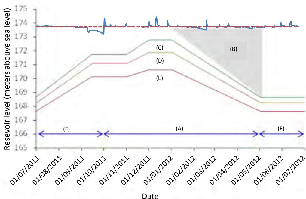
Figure 7. Maitai Reservoir water level for 1 July 2011 June 2012 super-imposed upon a graph of rules for operation of the water supply system. See the text below for a description of the lines and letters on the graph.
