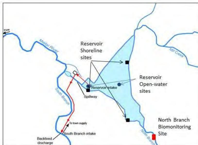
Figure 1. Diagram of the Maitai Water Supply Scheme with the water supply intake (labelled 'South Branch intake') and backfeed to the Maitai South Branch shown. Also shown are the Maitai Reservoir open water (blue-circles) and shoreline (black squares) sites, and the North Branch biomonitoring site (red rectangle) where sampling for water chemistry, macroinvertebrates and fish occurred.
