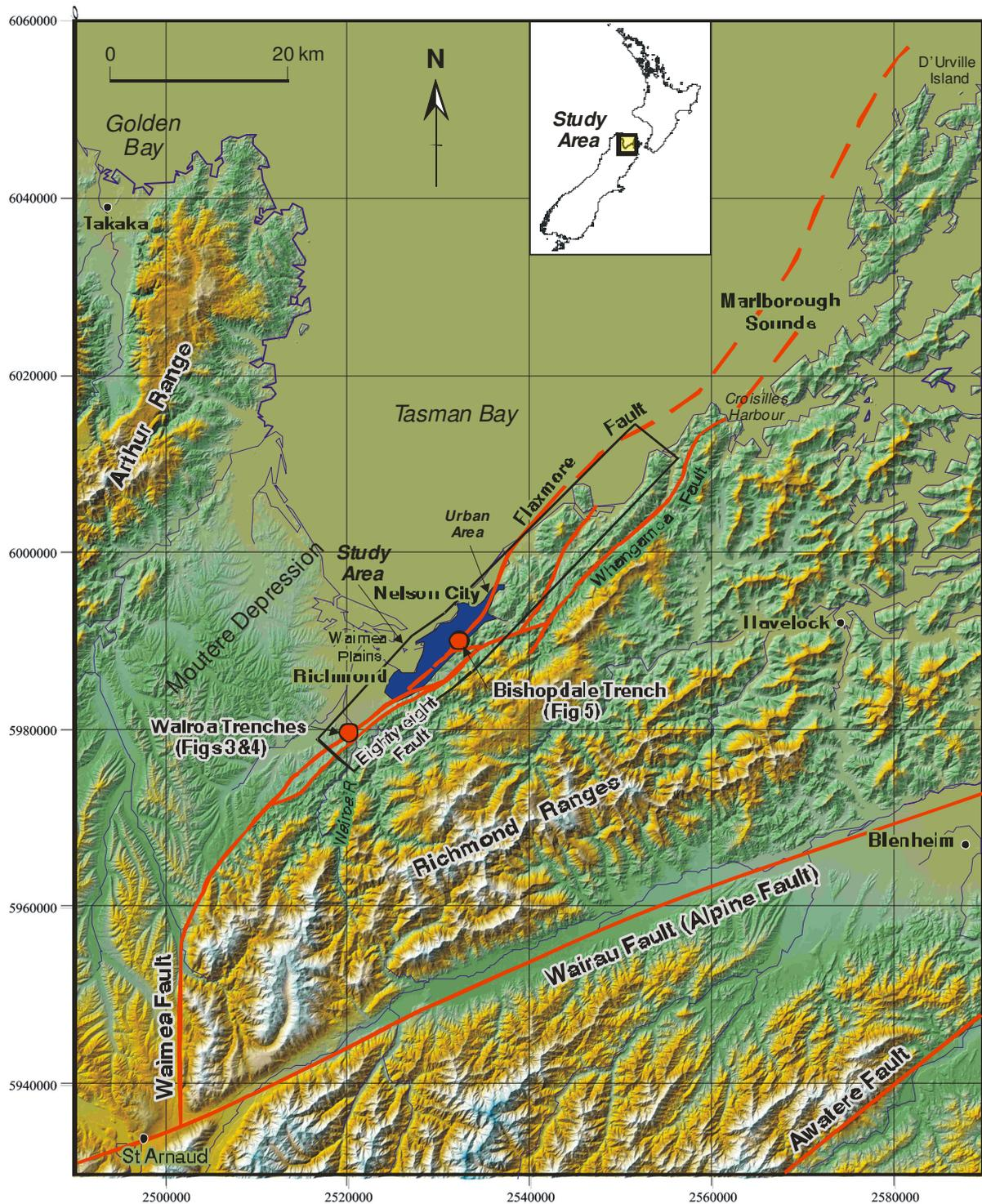
**Figure 1** Digital elevation model showing the location of the Waimea-Flaxmore Fault System (which includes the Waimea, Flaxmore, Eighty-eight and Whangamoa faults) relative to the main urban areas of Nelson and Richmond. Locations of Figure 3 and the trenches (Figures 4 & 5) are shown. Figure modified from Fraser (2005).
