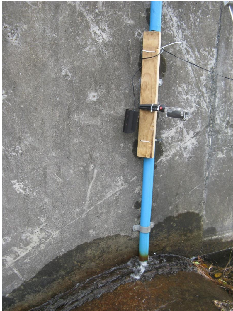
Figure 53. Infra-red time-lapse video camera at the Maitai Dam spillway crest, intended to monitor fish passage.
