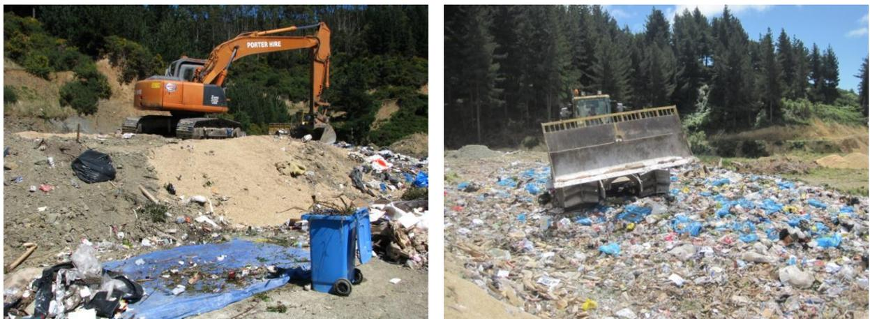
**Figure 3-4: Excavator and compactor used at York Valley Landfill**
